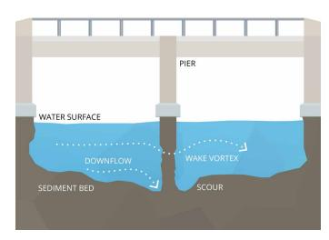
When sediment transport removes material from a streambed or bank, the erosion process is called scour. Scour can occur anywhere that there is water flow and erodible material. Local scour is the engineering term for the isolated removal of sediment at one location, such as the base of underwater structures, including bridge piers and abutments. This localized erosion can cause structural failure, as bridges and overwater constructions rely on the bed sediment for support.
