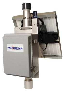
The iSIC-MAST system includes the data logger and solar panel premounted to a 2" diameter pole to create a truly plug-and-play data collection and sensor interface platform. The system integrates a NexSens iSIC data logger and 20-watt solar power kit - all in a compact, pre-configured package. Simply thread the system to any 2"NPT male pipe thread, connect the solar panel & battery, wire the sensors, and setup a project using iChart software - it's that simple!
